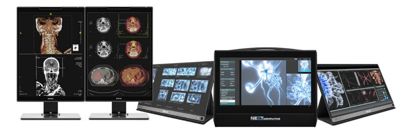
The RadStation by NextComputing is a portable multi-screen PACS radiologist reading station. It is an all-in-one solution, purpose-built and performance-optimized with the right combination of specs and tools for fast and accurate analysis of diagnostic scan files from X-rays, MRI, CT, Ultrasound, PET CT, and Nuclear Medicine.
